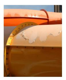
many years, UV exposure can deteriorate the gel coat surface and expose the structural fiberglass layers potentially reducing the structural strength of the fiberglass parts.
